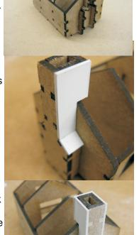
The sides and the end with windows in it are made up of 2 parts. Glue these parts together using a solvent such as plastic weld making sure there is an equal amount of space at the sides and that the bottom of the two pieces is flush.
